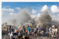
E-waste processing in Agbogbloshie, Ghana using open-burning of electronics to access valuable metals like copper. Open burning of plastics is common in many parts of the world without the capacity for processing. Especially without proper protections, heavy metals and other contaminants can seep into the soil , and create water pollution and air pollution .
