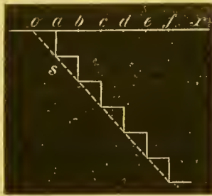
Fig. 109. s , Line of elasticity of an inorganic solid, such as india-rubber, indicating effects of equal increments of weight applied at a, b, c, d, e, f ; o x , abscissa (see text). (Marey, slightly altered.)
