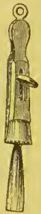
Fig. 119. Sartorius muscle of frog suspended by Kronecker's clamp, for experiments on chemical stimulation.
