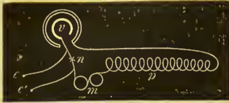
Fig. 118. Arrangement of the primary circuit when the extra stream is used as a stimulus. (Brücke.)
