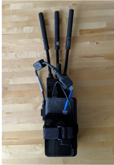
Figure 50. MPU5 Bundle (MPU5, External Battery, and Raspberry Pi)
