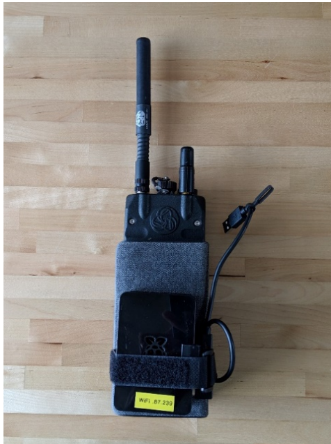
Figure 26. MPU4 Connected to the SNMP Agent via Wi-Fi without the 10/100 Ethernet Cable
