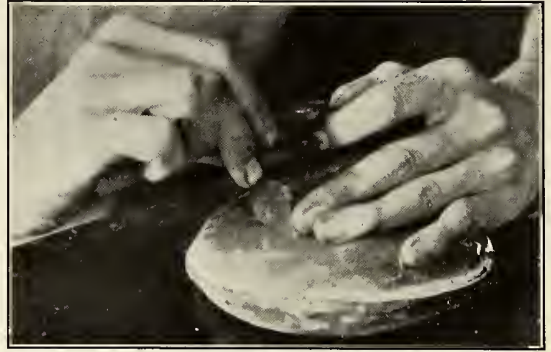
ENGRAVING THE PIN HEAD. Mr. Stuart's hands resting on a thick, leather cushion as he cuts the pin head with an ordinary engraver's tool.
