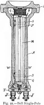
the object is to strengthen the field in which the diaphragm vibrates, by presenting both magnet poles to the diaphragm. The length of the path of the lines of force through the air is thus greatly shortened, and the field of force is concentrated at the point where it will be most effective.
