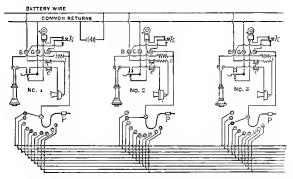
Fig. 215.—Common-Battery House System.
