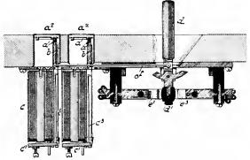
Fig. 207.—Supervisory Signals for Scribner System.
