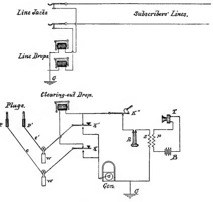
Fig. 133 .- Switch-Board for Grounded Lines.
