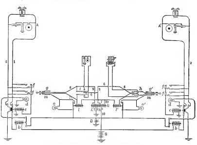
Fig. 209.—Scribner Multiple-Board System.
