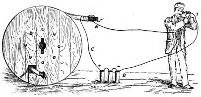
Fig. 340.--Receiver Test for Crosses and Grounds.
