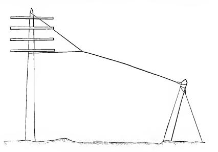
Fig. 296.-Guy Stub and Anchor.
