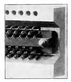
Fig. 239.—Line Terminals, Ford & Lenfest Distributing Board.
