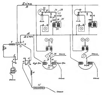
Fig. 253.—Reid & McDonnell Bridged Step-by-Step System.
