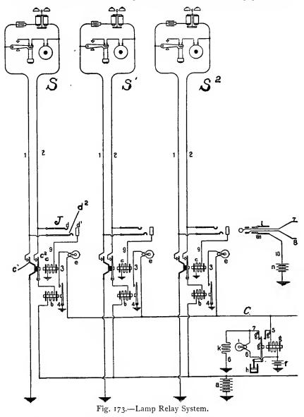
at the central office to pass through it and operate the call-bell in the usual manner. The high impedance of the call-bell magnets, however, prevents the short-circuiting of the voice currents
