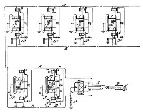
Fig. 262.—Circuits of Six-Station B. W. C. System.
