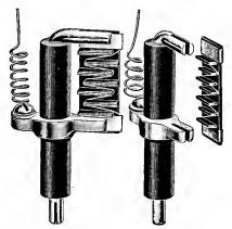
Fig. 322.—Fused Terminal Block for Moon Head.
