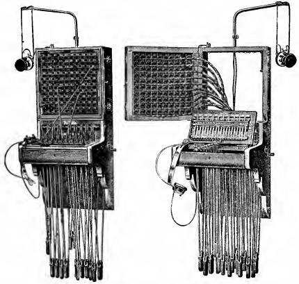
Figs. 165 and 166.—" Western " 100-Drop Wall Switch-Board.
