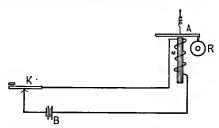
Fig. 4.-Morse Electromagnetic Telegraph.
