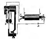
Fig. 47.—Double Transmitter.
