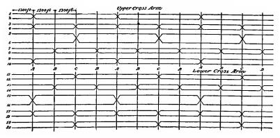
Fig. 124.-Diagram of Transpositions.
