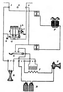
Fig. 89.-Complete Circuits of Bridged Telephone.
