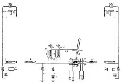
Fig. 206.—Scribner Common-Battery System for Small Exchanges.
