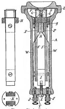
Fig. 23.—Bipolar Receiver.
