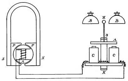
Fig. 70.—Diagram of Generator and Bell.
