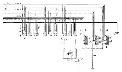
Fig. 176.—Diagram of Branch Terminal Multiple Board.
