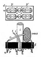
Fig. 235.—Detail of Connection Strips.
