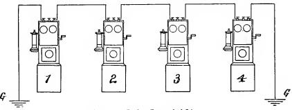
Fig. 243.—Series Grounded Line.
