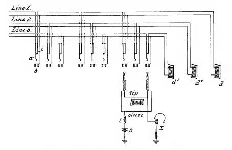
Fig. 174.—Simplified Diagram of Series Multiple Board.
