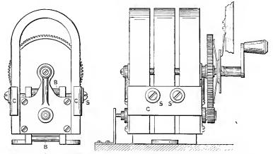
Figs. 93 and 94.-Details Western Telephone Construction Co. Generator.
