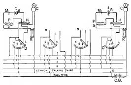
Fig. 218.—Diagram of Holtzer-Cabot System.
