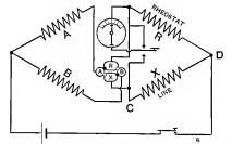
Fig. 345.-Circuits of Portable Testing Set.
