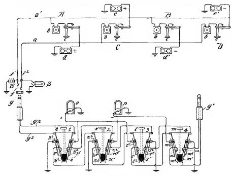
Fig. 257.—Hibbard Four-Station Line.
