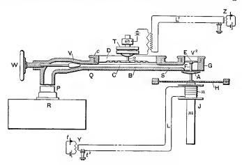
Fig. 115.—Erdman Telephone Relay.
