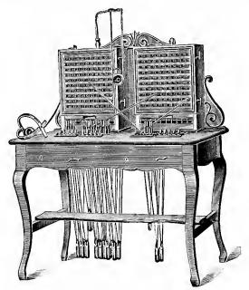
Fig. 168.—" Western " 200-Drop Table Switch-Board.
