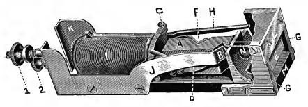
Fig. 160.-Western Telephone Construction Co.'s New Drop and Jack.
