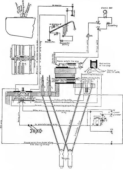
Fig. 167.—Circuits of "Western " 100-Drop Board.
