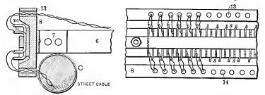
Fig. 238.—Line Terminals, Ford & Lenfest Distributing Board.
