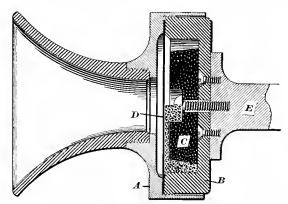
Fig. 43.-Western Telephone Construction Co.'s Transmitter.
