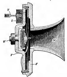
Fig. 39.-Sectional View Solid Back Transmitter.
