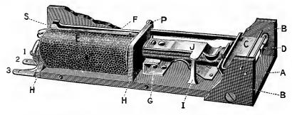
Fig. 158.—Western Telephone Construction Co.'s Drop and Jack.
