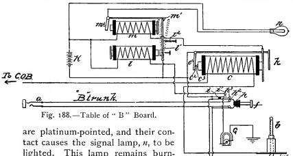
tact causes the signal lamp, n, to be lighted. This lamp remains burning until the called subscriber takes his telephone off the hook, which act closes the circuit through the combined clearing-out relay and signal, c,
