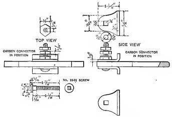
Fig. 64.-Details of Clamp for "Standard " Fuller Cell.
