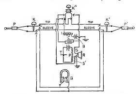
Fig. 175.-Cord Circuit of Series Multiple Board.
