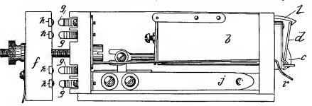
Fig. 161.—Side Elevation American Drop and Jack.
