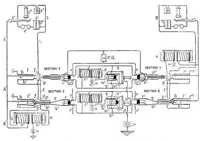
Fig. 178.—Complete Circuits of Branch Terminal Multiple Board.
