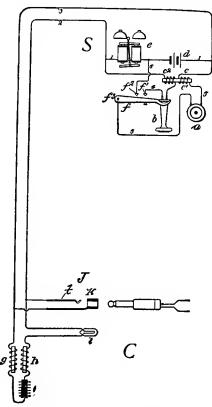
Fig. 172.—Lamp Signal System.
