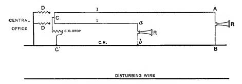
Fig. 127.—Induction on Common-Return Lines.
