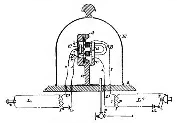
Fig. 116.—Stone Telephone Relay.
