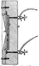
Fig. 20.—Hunning's Granular Carbon Transmitter.
