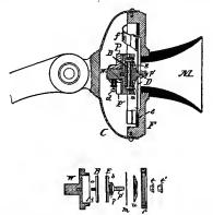
Fig. 38.-Details of Solid Back Transmitter.
