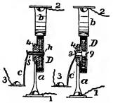
Fig. 224.—Details of Hayes Arrester.
