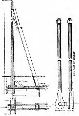
Fig. 292.-Details of Anchor Pole, and Guy Rod.
