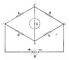
Fig. 342.--Diagram of Wheatstone Bridge.
