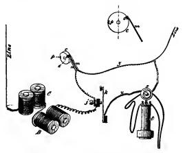
Fig. 250.—Line Circuit through Apparatus.
