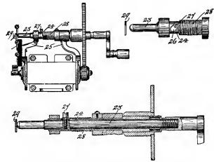
Fig. 77.—Details of Cook Armature Shunt.
