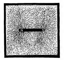
Fig. 2.-Lines of Force of Bar-Magnet.
