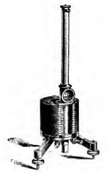
Fig. 346.-D'Arsonval Galvanometer.
