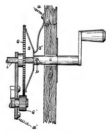
Fig. 76.-Western Telephone Construction Co. Armature Shunt.
