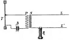
Fig. 21.-Transmitter with Induction Coil.
