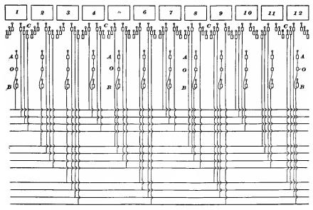
Fig. 189.—General Scheme of Western Transfer System.
