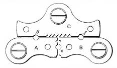
Fig. 219.—Usual Form of Telephone Lightning Arrester.
