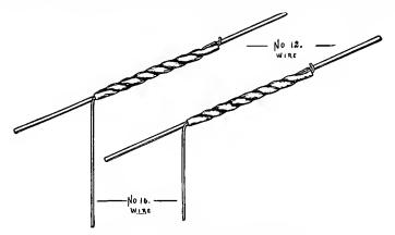
Fig. 308.—Branch Wires with Lillie Joint.
