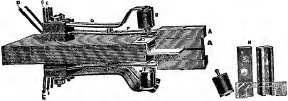
Fig. 228.-Combined Carbon and Heat Coil Arrester.
