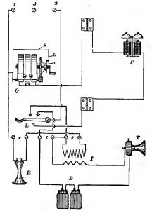
Fig. 87.-Complete Circuits of Series Telephone.
