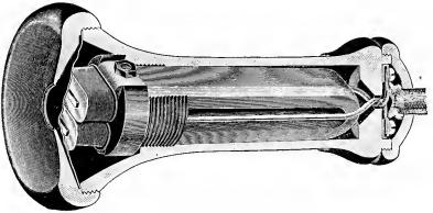
Fig. 25.-Western Telephone Construction Co.'s Receiver.
