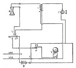
Fig. 90.—Circuits of Battery Call Instruments.
