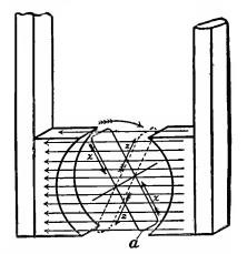
Fig. 68.—Field of Force in Magneto-Generator.
