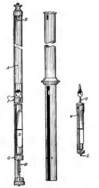
Fig. 347.—Suspension of D'Arsonval Galvanometer.
