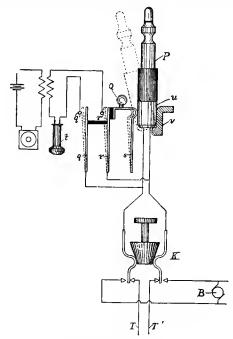
Fig. 153.—Plug Socket Listening Key.
