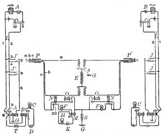
Fig. 208.—Hayes System as Applied to Multiple Boards.
