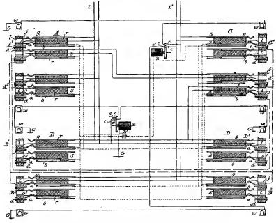
Fig. 184.—Kellogg Divided Multiple Switch-Board.
