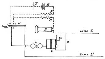
Fig. 79.--Telephone Circuits, Hook Down.
