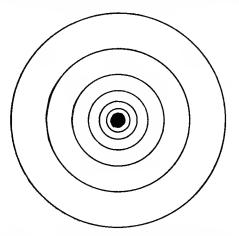
Fig. 117.-Magnetic Lines around a Conductor.
