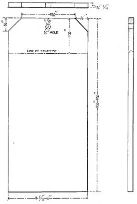
Fig. 63.-Carbon Plate for "Standard " Fuller Cell.
