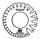
Fig. 268.—Circular Wire Gauge.
