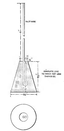
Fig. 65.—Zinc for "Standard" Fuller Cell.
