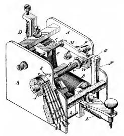
Fig. 249.—Dickerson Step-by-Step Mechanism.
