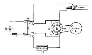
Fig. 353.-Connections for Insulation Test.
