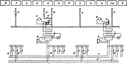
Fig. 190.—Transfer and Instruction Circuits.
