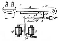
Fig. 248.—Busy Signal for Lock-out System.
