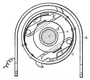
Fig. 78.—Williams Armature Shunt.
