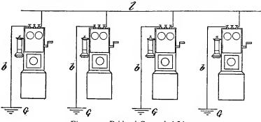
Fig. 244.—Bridged Grounded Line.
