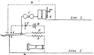
Fig. 81.-Telephone Circuits, Hook Down.
