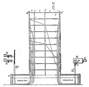
Fig. 230.—End View Hibbard Distributing Board.
