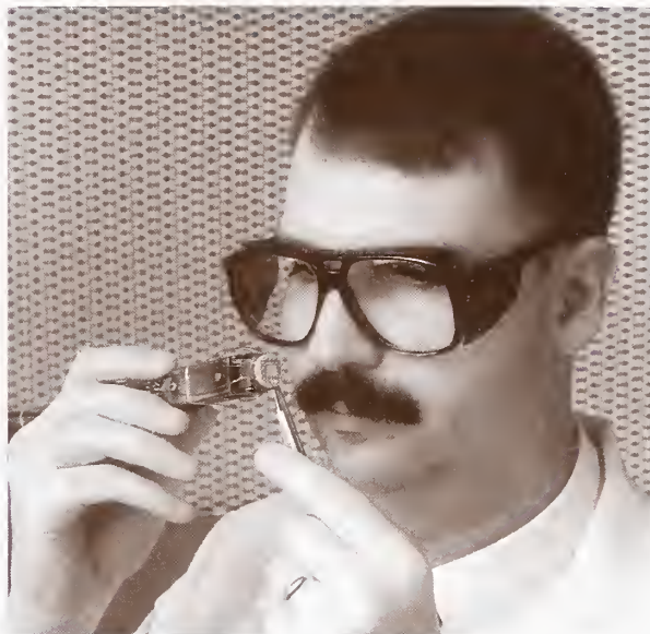
LOADING SILICON DEVICE ON TILTING SAMPLE STAGE FOR INTERFACE ROUGHNESS MEASUREMENTS
