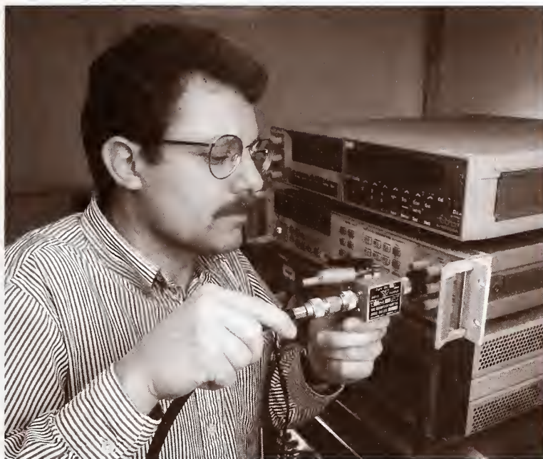
VERIFYING AN AC VOLTAGE POINT ON THE MCS
