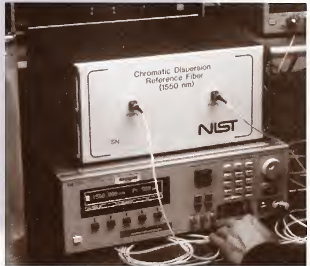
DEVELOPMENT OF STANDARD REFERENCE MATERIAL (UPPER BOX) SRM will support systems for determining dispersion properties of optical fiber, in particular, the zero-dispersion wavelength
