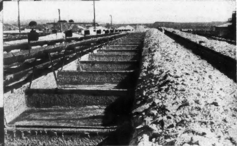
Right: Crystallizing tanks with crystallized nitrate removed to shelves where it is allowed to drain, after which it is moved in a small car to storage piles. Tanks are ready for another charge of 60 per cent nitrate solution.
