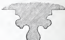
Fig. 1097. Transverse and Diagonal Rib; and Wall Rib—CHOIR A FOUNTAINS ABBEY, VAULTING RIBS
