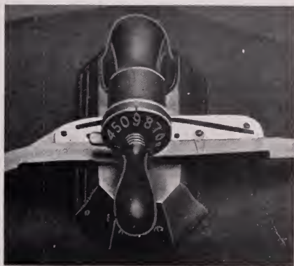
Fig. 1—Showing the check perforating machine fitted with a track which will take a strip of tin foil three quarters of an inch wide. On the left hand side the foil has already been perforated, while on the right hand side no perforation has been made.
