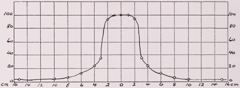
Fig. 18. Influence of Secondary Radiation on the Distribution of the Dose within and without the Radiation Field, Measured in Water, Size of Field 4x4 cm. Roentgen Rays filtered through 1 mm. Cu.
