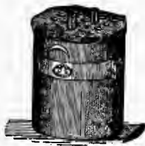
FIG. 22—WASTE-JAR FOR EMPTYING TEST-BOTTLES
