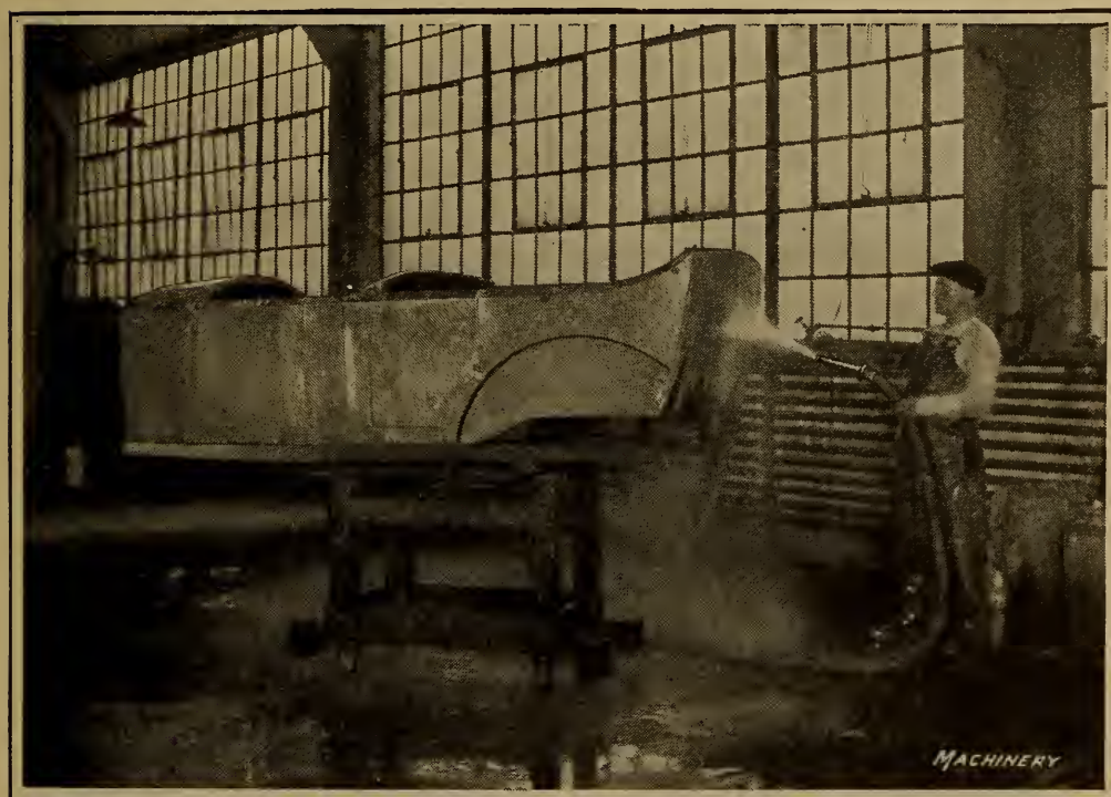
Fig. 2. Washing Car Body to remove Alcohol and Surplus Deoxidine
