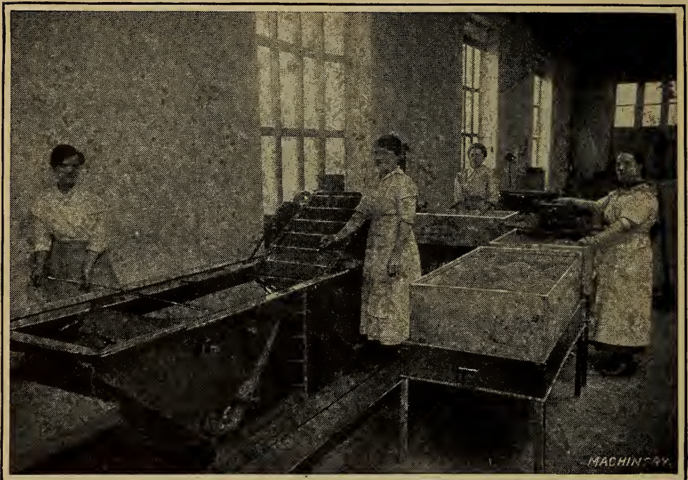
Fig. 5. Oil Tank in which Bodies are dipped to produce Rustproof Coating
