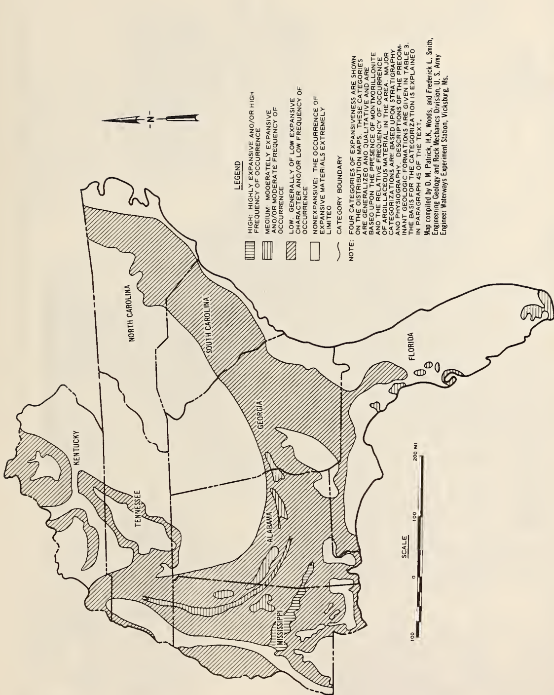
Figure 3. Distribution of potentially expansive materials in the United States; FHWA Region 4
