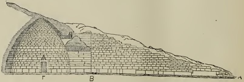
Fig. 43. Section of "Treasury of Atreus"
