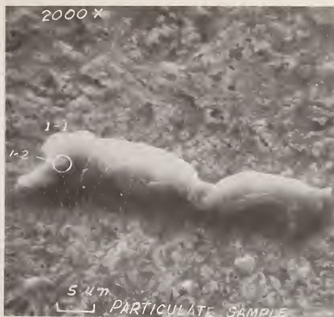
Figure 11. Impactation region from rocket plume 2,000 X SEM.
