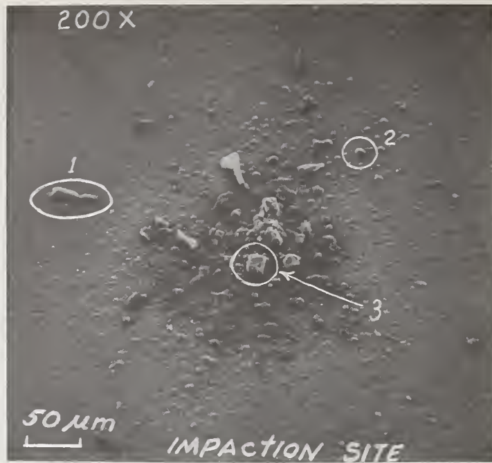
Figure 9. Impactation region from rocket plume 200 X SEM.
