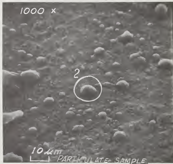
Figure 10. Impactation region from rocket plume 1,000 X SEM.
