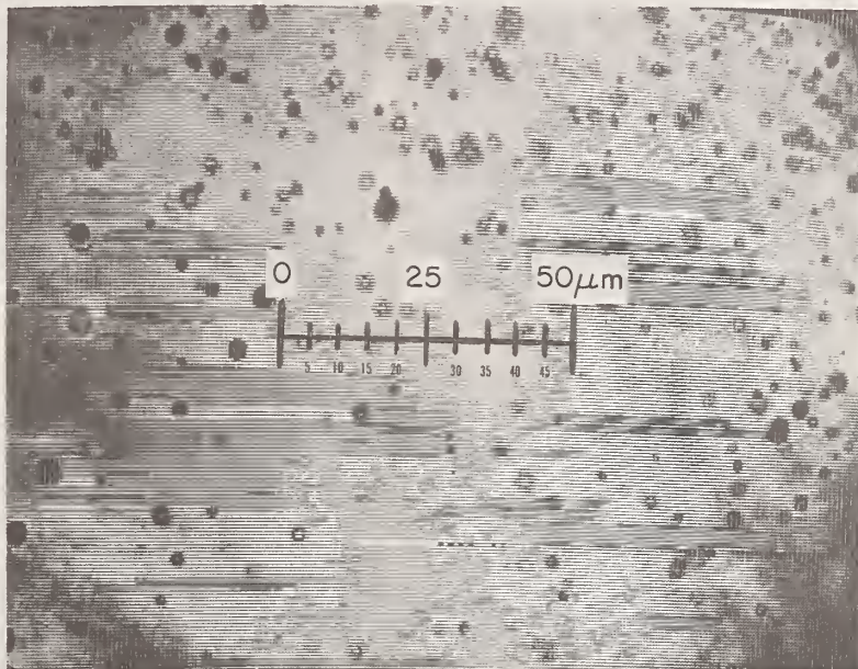
Figure 18. Frame taken 20 cm downstream from nozzle shows particles in free flight.
