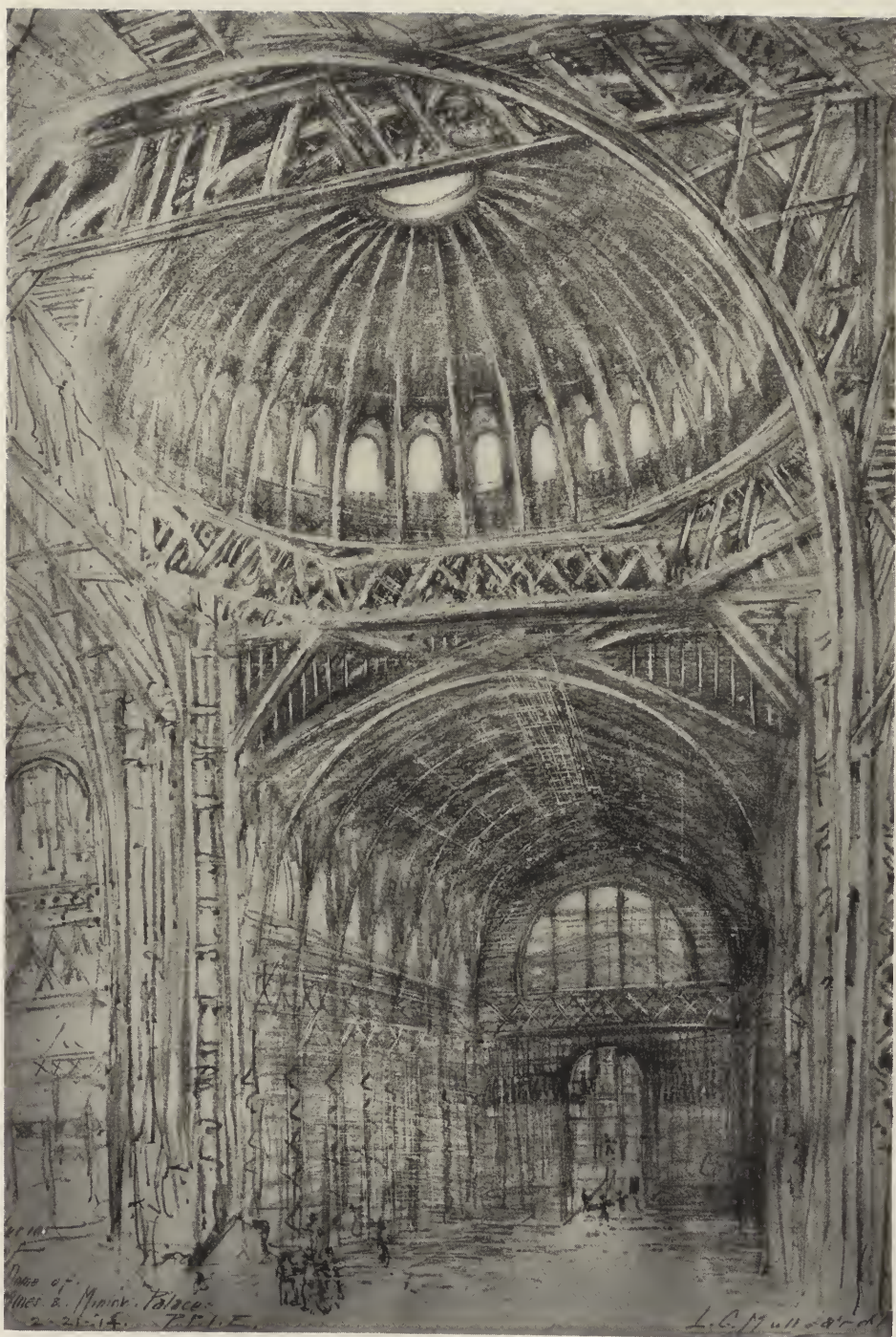
SKETCH OF TYPICAL INTERIOR CONSTRUCTION OF THE EIGHT DOMES AS DESIGNED BY THE ENGINEERING DEPARTMENT OF THE PANAMA-PACIFIC EXPOSITION: BLISS & FAVILLE, ARCHITECTS.
