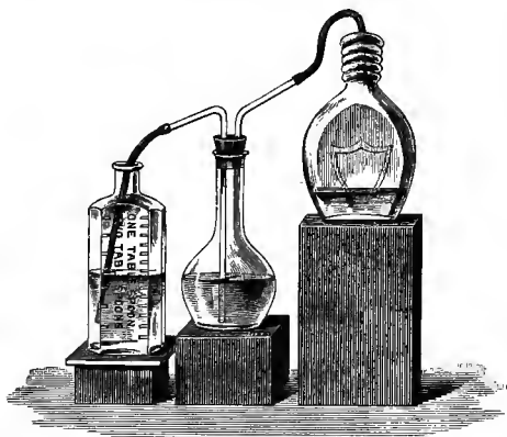
Fig. 3.—APPARATUS FOR ESTIMATING DIABETIC SUGAR BY FERMENTATION.
