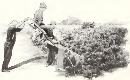
L-blade root pruner. Starting blade at the end of a row of White Pine trees, it cuts the tap root and the side roots on one side. Next year it can be used on the other side
