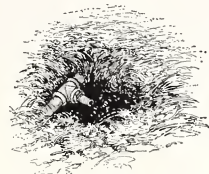
9. Why the trees grow. A water pipe, below the ground. The gardener said, "If it is on top of the ground it interferes with mowing. We plowed a furrow and put it underground. We know the lowest point and drain it out in the winter. At this 'T' we can attach a hose"
