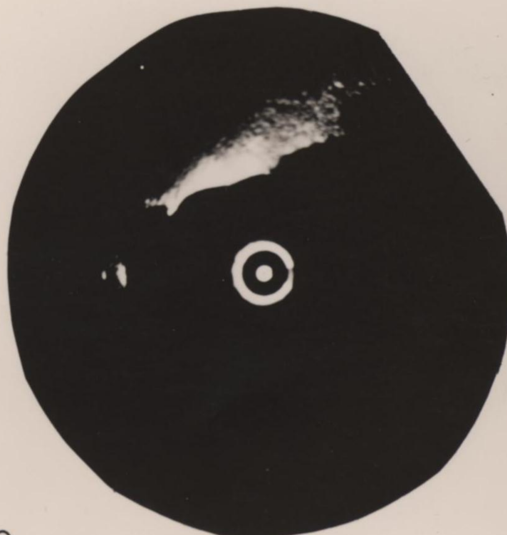
20 MILE SWEEP PLANE BANKING, SHOAL POINT AT 12 O'CLOCK ROCKY POINT AT 9 O'CLOCK
