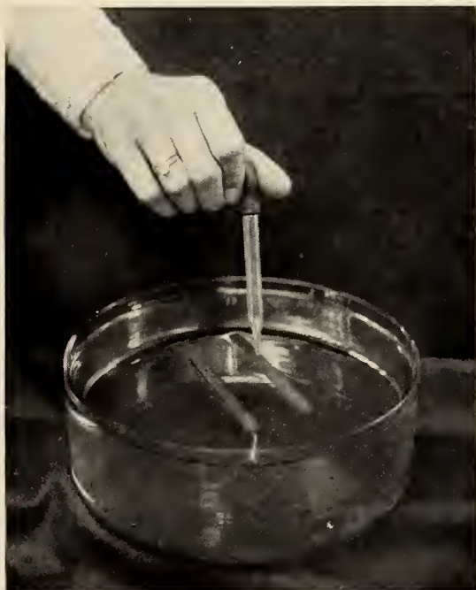
DROPPING ALCOHOL BETWEEN TWO STICKS TO WEAKEN THE SURFACE FILM OF THE WATER.
