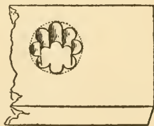
Fig. 168. Drilling the Mast Step.
