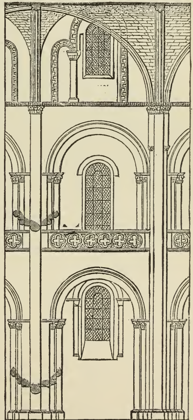
382. Elevation of Compartment of Nave of St. Stephen, Caen. (From Pugin.)
