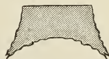
139. Section of half of the Ionic Capital at Bassæ, taken through the volute.
