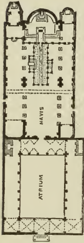
273. Plan of the Church of San Clemente at Rome. (From Gutensohn and Knapp.) 2 Scale 100 ft. to 1 in.
