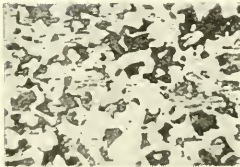
FIG. 3.—SECTION OF GOOD RAIL.
