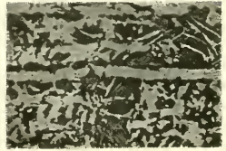
FIG. 5.—SECTION OF RAIL AFTER ROLLING.
