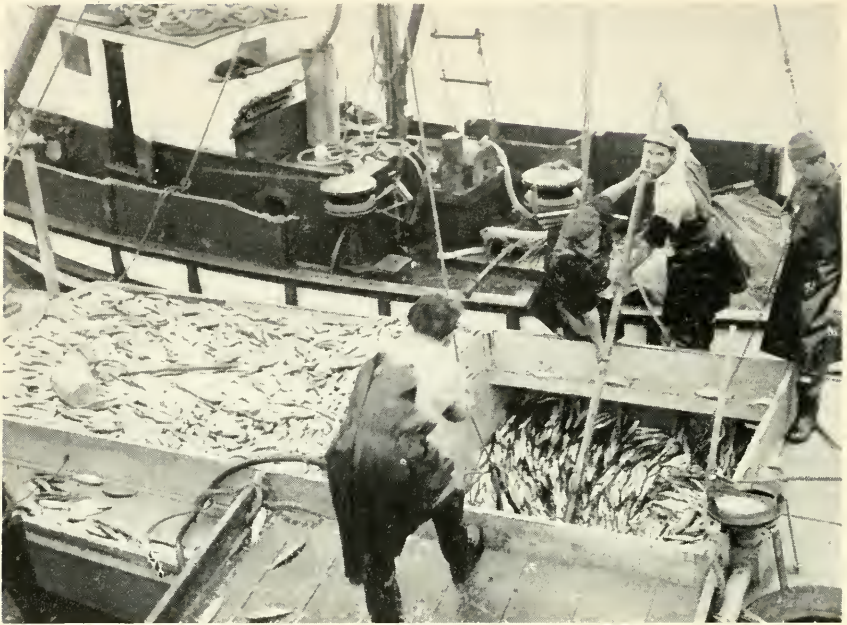
FIGURE 62. Unloading sardines from the barge of the lampara boat SAL BOY, at a Moss Landing cannery. The fifth man of the crew, not in photo, is operating a hoisting winch. Note the net-pullers mounted on the deck of the powerboat. Photograph by J. B. Phillips, September 18, 1950.
