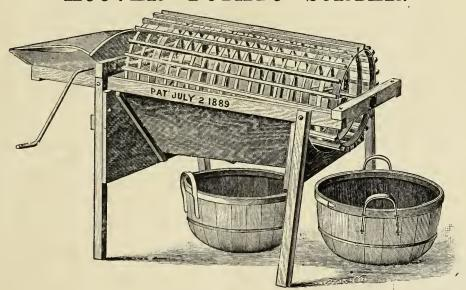
The above cut represents the Hoover Potato Sorter. You will notice at once that it is "just the thing." "Wonder some one has'nt thought of it before." With this Machine which weighs less than 100 pounds, two men and a boy can sort and put in the wagon from 80 to 100 bushels an hour. For prices, etc., address
