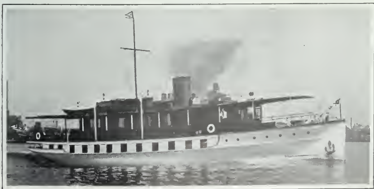
Alscotia , a 98½-foot houseboat owned by Mrs. Stricker Coles, at Essington, Pa. She was built by Mathis and is powered with two Winton gasoline engines
