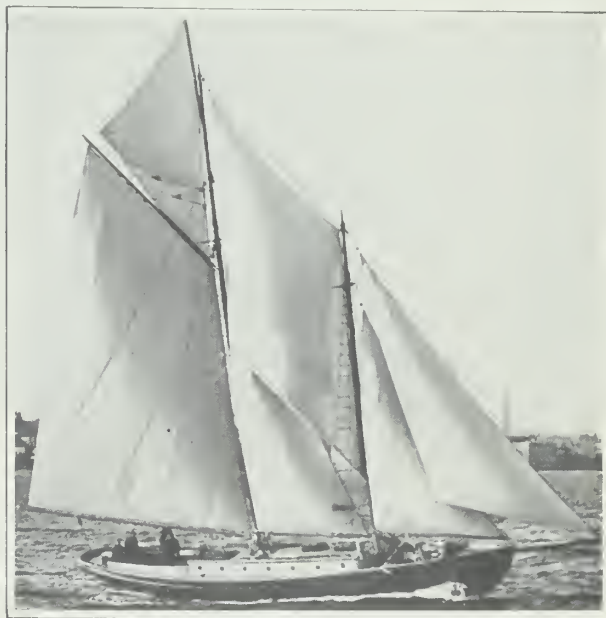
Tigress , a 56-foot schooner yacht designed by William H. Hand, Jr., and built by Hodgdon Brothers. An auxiliary motor gives her a speed of ten miles under power
