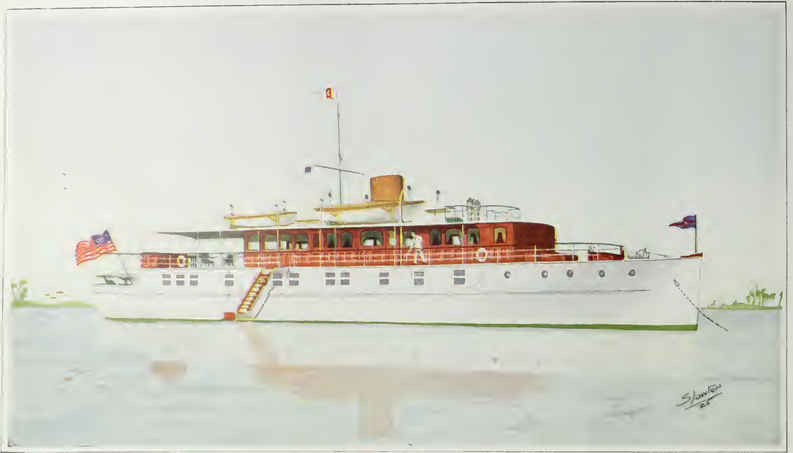
The new motor yacht built by Ditchtown Boats, Ltd. for Mr. J. H. R. Cromwell is considerably larger than the Pyne boat (being 90 feet over all), but still shows a tendency for speed. She is powered with two 350 h. p. Winton engines which develop a speed of twenty miles per hour. Designed by Tams & King
