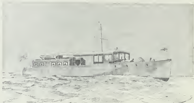
Another and smaller motor yacht, Brook II , designed by Tams & King and built at Petersen's Yard for Mr. Percy R. Pyne, II. Being essentially a commuting boat, she is equipped with two 225 h. p. Sterling motors which give her a speed of twenty-seven miles per hour; but she is also large enough (58 feet overall) to be thoroughly seaworthy for ordinary coastwise work, with comfortable sleeping accommodations for two
