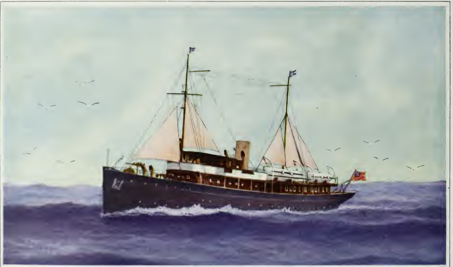
Mr. Harry Payne Bingham's auxiliary yacht Pawnee, designed by Cox & Stevens, is large enough for ocean cruising, measuring 160 feet over all and powered with Winton engines of Diesel type. She is more than a pleasure craft however, being equipped for fishing and for deep sea soundings, and having a complete marine laboratory for scientific research
