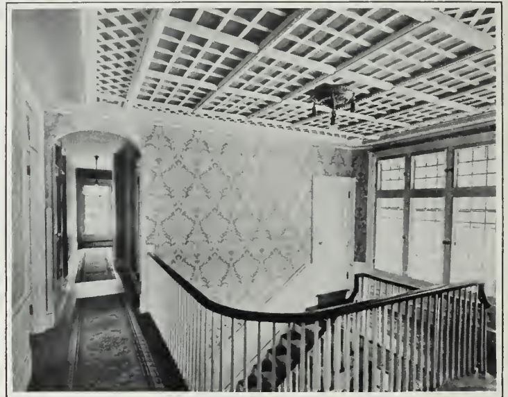
A woodwork design makes a decorative ceiling and screens the tone outlet, which is covered with thin cloth. The installation of the organ proper is in the attic, the keyboard on the main floor
