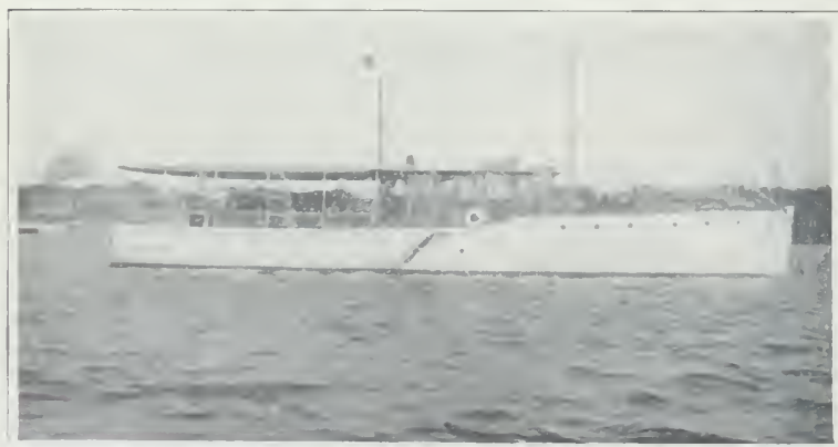
The Valia , a 70-foot yacht owned by Mr. Richard E. Traiser, at Boston, Mass. It was designed and built by F. S. Nock, and is powered with two Sterling Coast Guard six-cylinder engines
