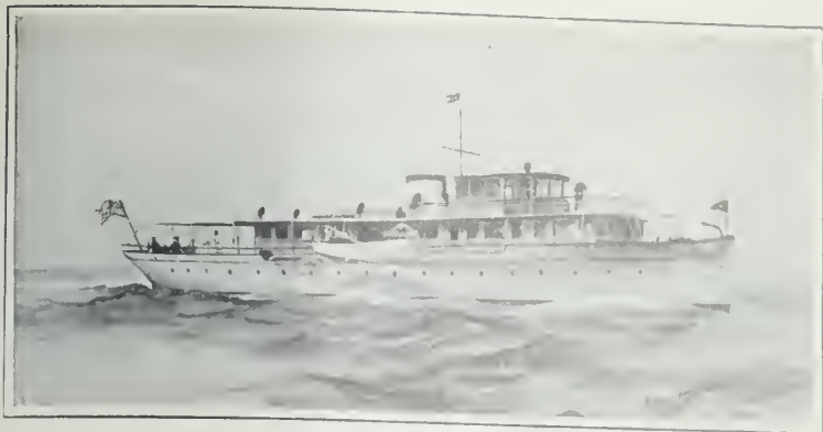
A notable addition to the New York Yacht Club's fleet is the Nevada , built at the Nevins Yard. Designed by Tams & King for Mr. D. H. Warner of Bridgeport, Conn., she is 110 feet over all and is of the coastwise and ocean going type of motor yacht, being equipped with two 140 h. p. Diesel motors with which she can make fifteen miles per hour or better
