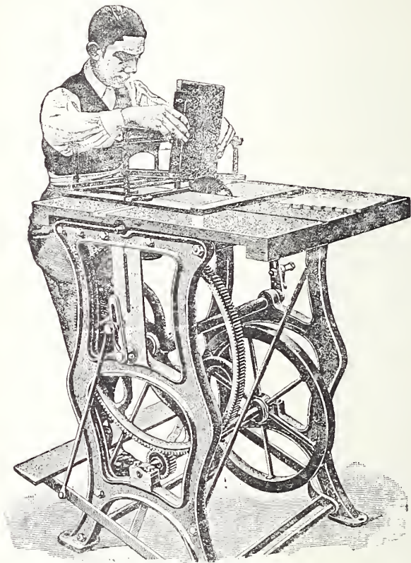
Fig. 76.—Circular Saw with Dovetailing Appliance.
