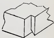
Fig. 90.—Dovetail Stopped Back from Front.
