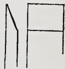
Fig. 71.—Properly Ground Edge.
