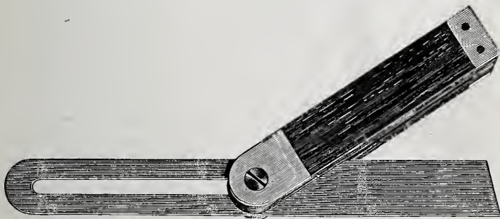
Fig. 33.—Improved Ebony Sliding Bevel.
