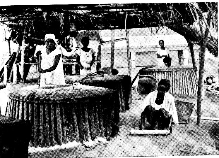
The brine is evaporated in the cauldrons over the furnaces.
