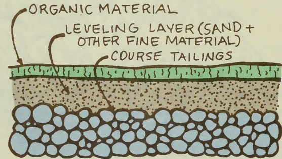
APPLICATION OF LEVELING LAYER + ORGANIC MATERIAL
