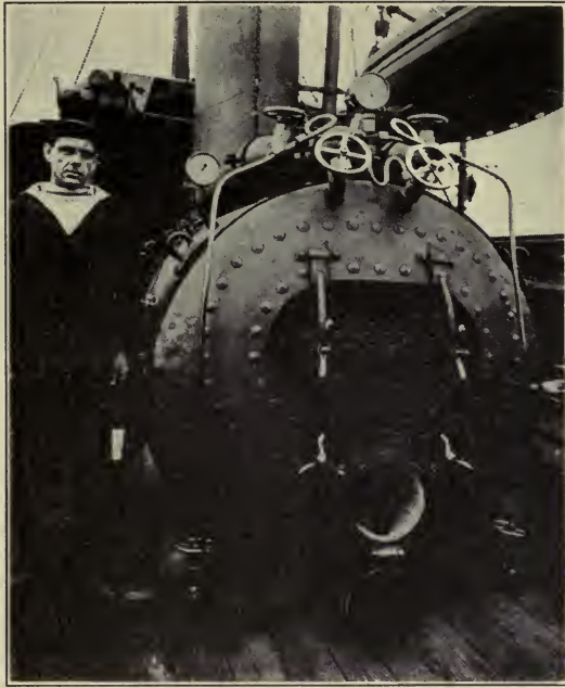
Figure 84. Outside of naval recompression chamber, showing man- hole for access, and air lock for food.
