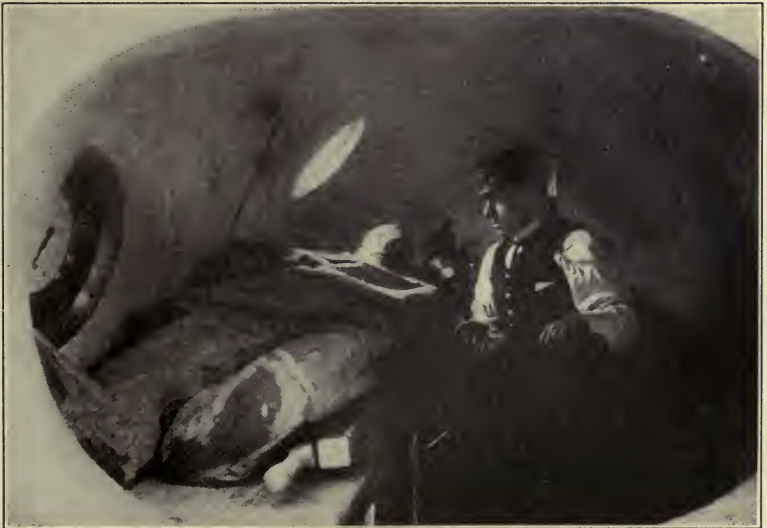
Figure 85. Inside of recompression chamber, showing bed for patient.
