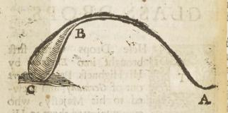
AB the thread, BC the body, B the neck, A the point or end of the thread.
