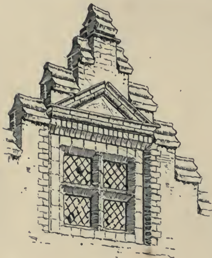
A WINDOW FROM NORFOLK IN MOULDED BRICK
