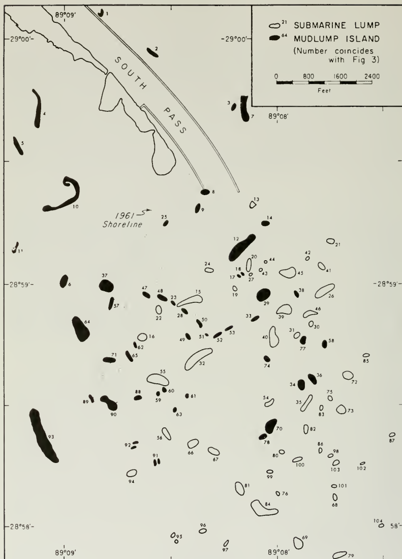
Text-figure 1. Mudlump distribution South Pass. Data from 123 maps dated between 1867-1961. (After Morgan, 1963, fig. 2.)
