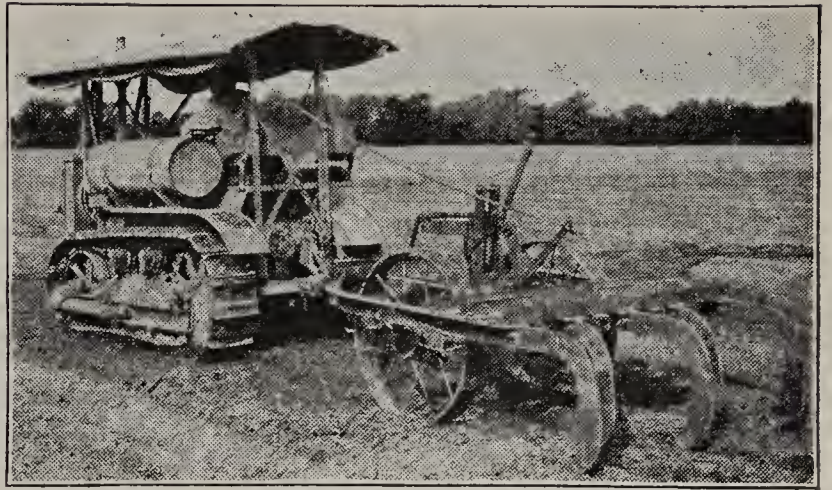
This specially designed chisel pulverizes soil 24 to 30 inches assuring perfect root systems.
