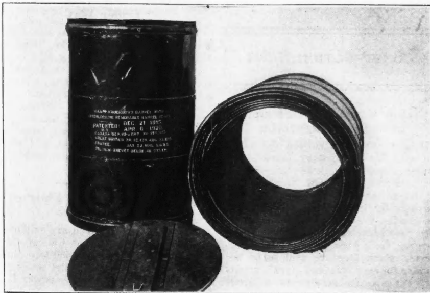
Sheets of seven barrels nested for shipment. Upright barrel contains heads and wires for seven barrels
