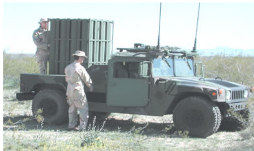
Figure 6. NLOS-LS Box Containing 16 Slots
