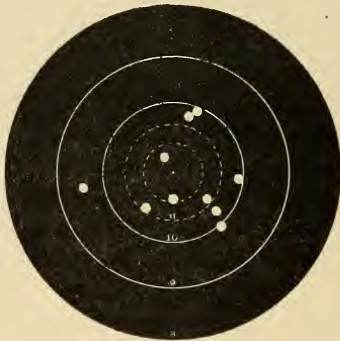
Fig. 78.— Ten shots at fifty yards by Mr. H. S. Harris. Shot at Walnut Hill, Mass., Jan. 6, 1894, with a Stevens Diamond Model Pistol with a ten-inch barrel and U. M. C. Co. .22 caliber, long-rifle cartridges.
