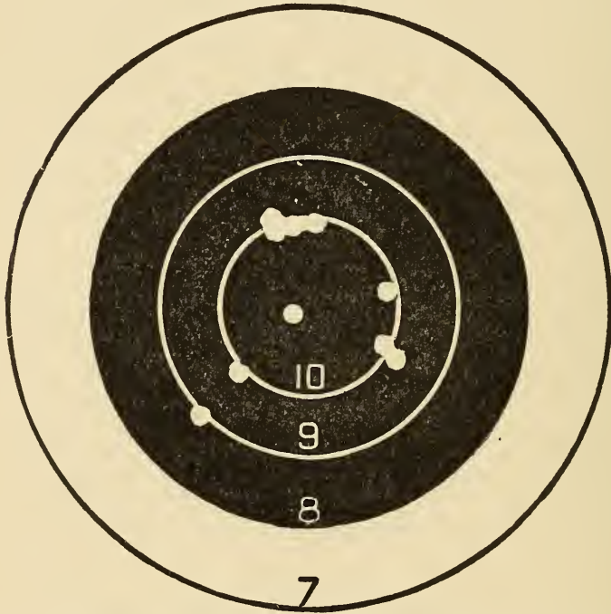
Fig. 101. — Ten shots by Mr. F. B. Crowninshield, at twenty yards, with a Wurfflein Pistol. Reduced from a bullseye 2 11-16 in. diameter.
