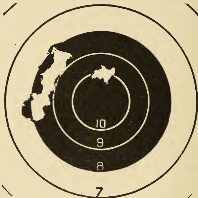
Fig. 86.— Five consecutive shots at twelve yards, with Smith & Wesson .38 caliber Pocket Revolver, 3\frac{3}{4} inch barrel.
