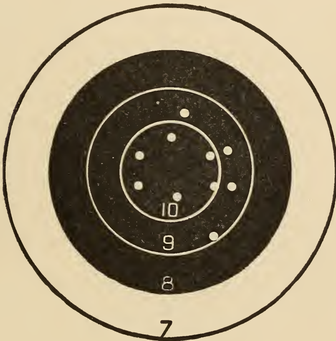
Fig. 111. — Ten consecutive shots at fifty yards, by Mr. F. B. Crowninshield, at Walnut Hill, Mass., June 4, 1892, with a Stevens Gould Model Pistol, .22 caliber; score 96. Target reduced to one quarter original size.
