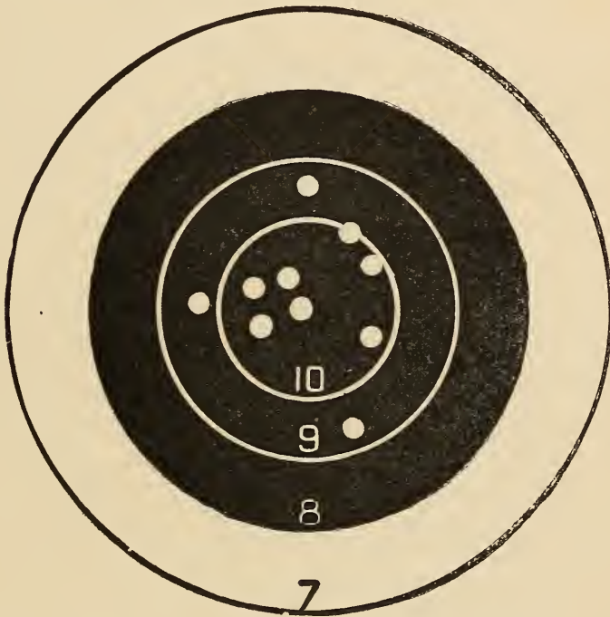
Fig. 43. — Ten shots at fifty yards by Mr. F. E. Bennett. Shot with a Smith & Wesson .44 caliber Russian Model Revolver with U. S. Cartridge Co's ammunition.
