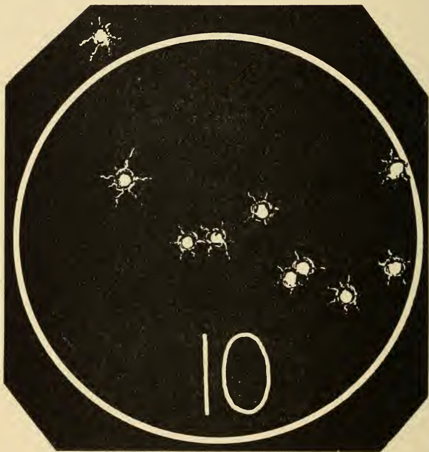
Fig. 109. — Score ninety-nine out of a possible hundred. Shot by Mr. Henry S. Harris, in Pistol Match of 1890, at Walnut Hill, Mass., with a Diamond Model Stevens Pistol and Union Metallic Cartridge Co.'s .22 caliber Long-Rifle Cartridges. Distance fifty yards; target full size. Highest score made during the year.
