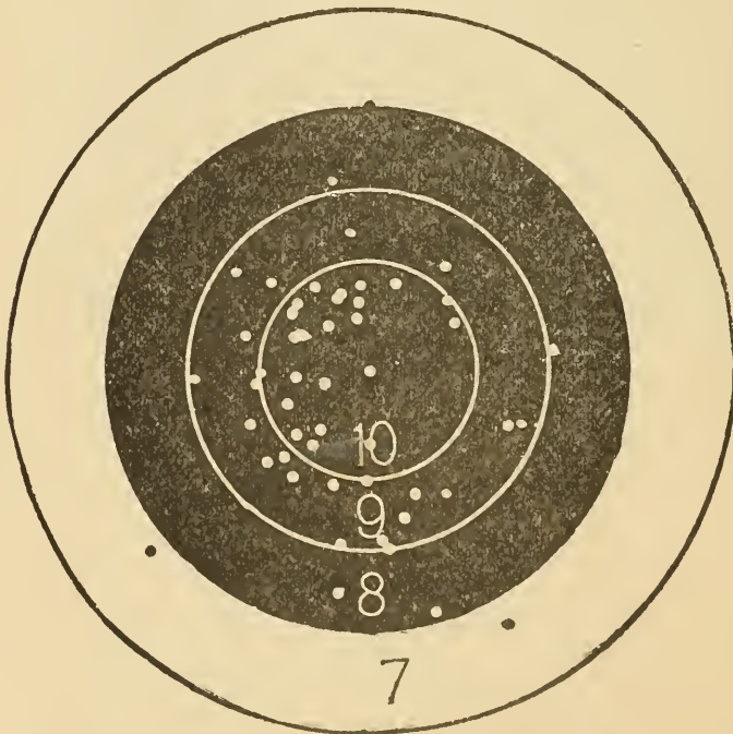
Fig. 10. — Fifty consecutive shots, at fifty yards, shot by Mr. J. B. Fellows, at Walnut Hill, Mass., with a Stevens .22 caliber pistol and U. M. C. Co.'s ammunition. Score, 456 points, shot on fifty yards pistol target.
