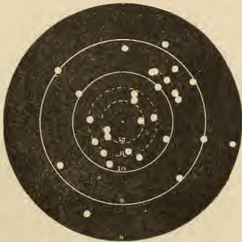
Fig. 90.—Thirty shots, by Mr. H. S. Harris, at fifty yards, with Stevens Gould Model Pistol, .22 long-rifle U. M. C. cartridge, at Walnut Hill, Mass., Dec. 30, 1893.
