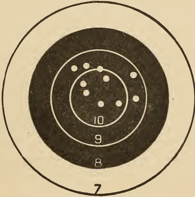
Fig. 117.—Ten shots at fifty yards, by Mr. H. J. Mehard, of Philadelphia, Penn. Shot with a Wurfflein pistol, Dec. 2, 1893. Score ninety-six. Reduced one quarter.
