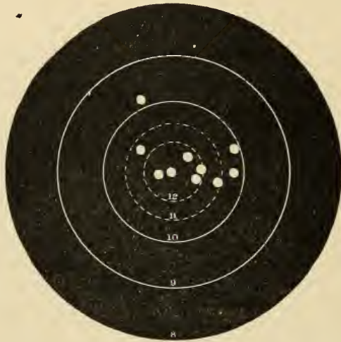
Fig. 77.— Ten shots at fifty yards by Mr. H. S. Harris. Shot at Walnut Hill, Mass, Dec. 31, 1890, with a Stevens Pistol, Diamond model with a ten-inch .22 caliber barrel. Ammunition, U. M. C. Co.'s long-rifle.
