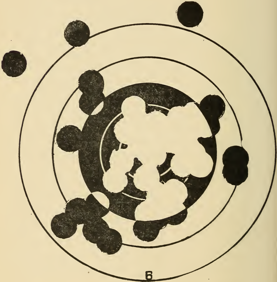
Fig. 80.— Fifty consecutive shots at twelve yards, by an ordinary marksman, with a Smith & Wesson .38 caliber Pocket Revolver, 3\frac{1}{4} inch barrel, U. M. C. Co., ammunition.
