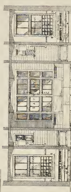
LONGITUDINAL SECTION THROUGH LAUNDRY, SCULLERIES AND W.C.
