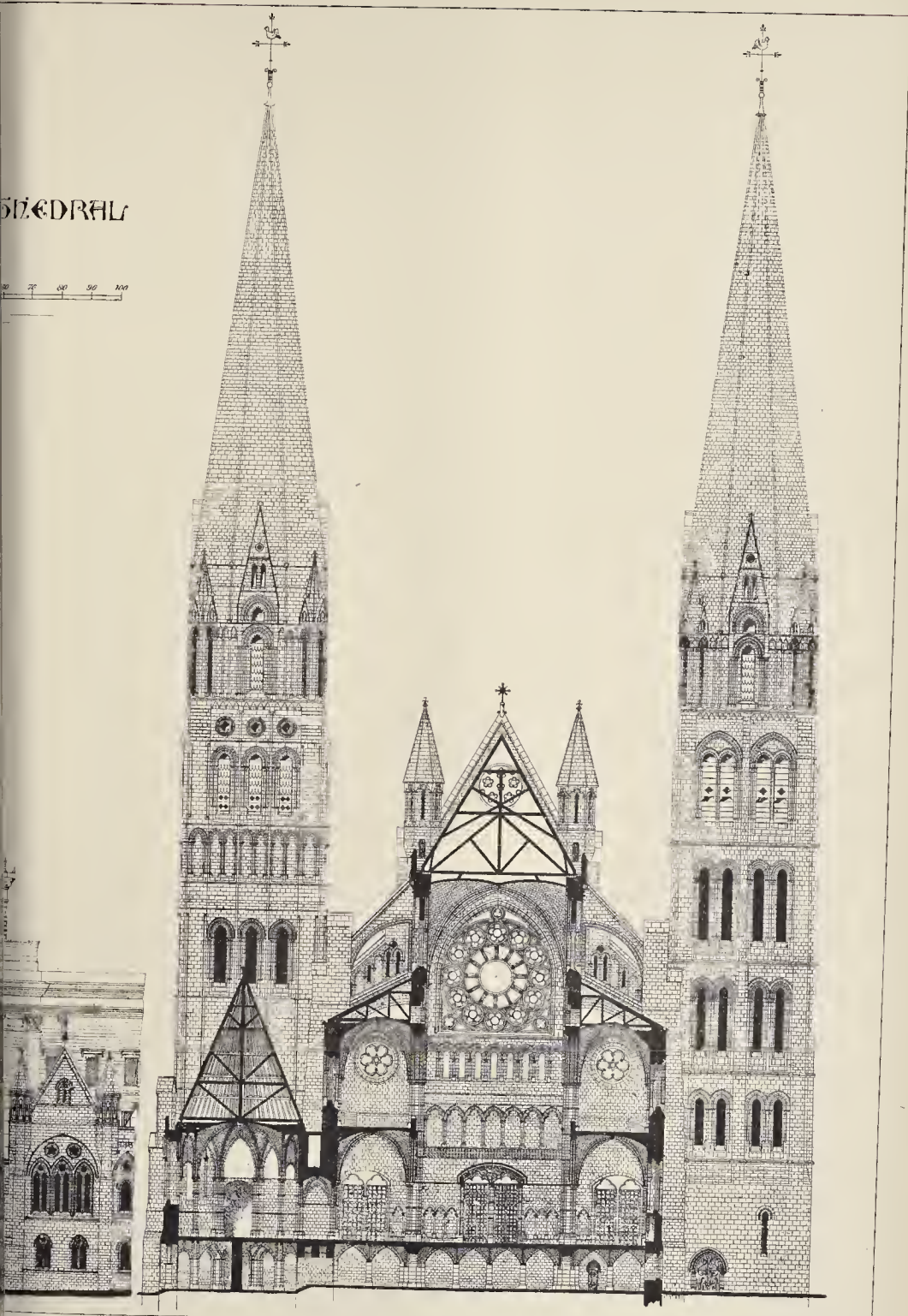
TRANSVERSE SECTION LOOKING WEST.
