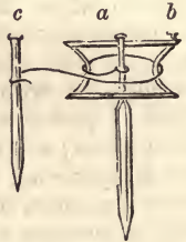
Iron reel and pin for a garden-line.
