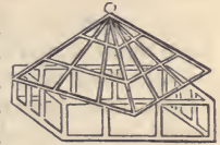
Cast-iron hand-glass in two parts, the roof and sides.
