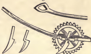
M'Intosh's wheel verge-cutter.
