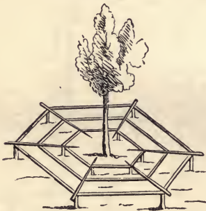
Isometrical view of the tabular tree-guard.
