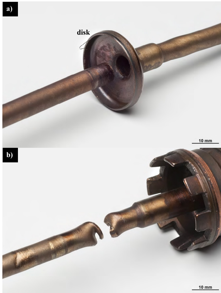
Fig. 14 Higher magnification photographs of the fracture locations a) 1 and b) 2
