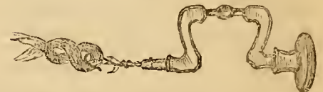
Fig. 5.—IMPLEMENT FOR TWISTING STRAW ROPE.
