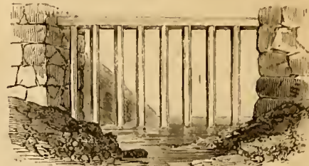
Fig. 5—PERMANENT WATER FENCE.
