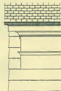
DETAIL of MAIN CORNICE
