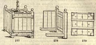
approved. Two of the opposite sides are fixed, the other two are moveable, but kept in their places by a couple of iron bars with hinges, which are fastened on one side, and on the other are hooks to catch in (fig. 177.), that the state of the roots may be readily examined, the old earth taken out, and fresh put in at pleasure. Another material advantage gained in these boxes is, that the plants may be shifted by sliding them into others.
