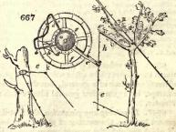
an inch on the wheel, and tells what exceeds the inch after a lesser spring (e), which strikes at every inch, has struck the bell. The circumference of the wheel (f) measures two feet. The rods for working the measuring machine are each three feet long, and one inch in diameter, with connecting screws of brass on each end of them; so that as many as are
