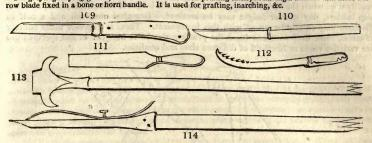
The budding-knife (fig. 110.) differs from the grafting-knife, in having the point of the sharp edge of the blade rounded off in the same manner as is the back or blunt edge of the grafting and pruning knives. It has also a thin wedge-shaped ivory or bone handle for raising up the bark, in the operation of inoculation.
