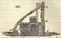
on moveable trellis-rods, composed of a centre and two side wires, and placed five feet apart; these rods are hinged to the front props, and supported in the middle of the roof, and at top, by chains and hooks, and in this way can be raised or lowered at pleasure. This house, since its erection, in 1817, has given the greatest satisfaction, and already pro-
