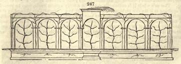
1574. Arched, niched, or recessed walls (fig. 247.) were contrived for the same purpose by Switzer, and, at least, had a massive imposing effect to the eye. Such walls were generally heated by flues, and formed in fact the intermediate link in the progress of im-
