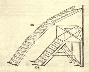
1461. The step-ladder (fig. 208.), instead of round rods on which to place the feet, has steps or boards, an improvement essentially necessary, where much work is to be done, because less fatiguing to the feet. Such ladders have a back or fulcrum by which they stand independently of any other object, and which is removeable at pleasure by drawing out an iron bolt.
