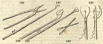
1354. The peach-gatherer (fig. 148.) consists of a tin funnel or inverted hollow cone, fixed on the end of a rod or handle at an obtuse angle, the funnel is first introduced under each fruit, and then gently raised or moved sideways; if ripe, the fruit will fall into the
