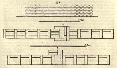
1562. Hollow walls may also be formed by using English instead of Flemish bond: that is, laying one course of bricks along each face of the wall on edge, and then bonding them by a course laid across and flat. Such a mode has been practised and described by Dearne, an architect in Kent.
