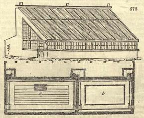
placed somewhat nearer to the roof. The name and character of this structure is derived from the higher degree of heat generally kept in it, and from the air being less moist than in the bark-stove, where more water is used, and consequently more vapor generated. The volume of air to be heated by one fire in the dry-stove, should not exceed two thirds of that to be heated in a green-house or conservatory, similarly constructed and situated.
