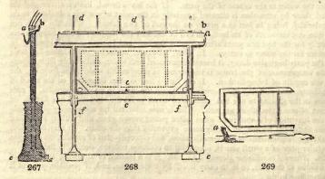
1642. Where the roof is moveable on the polyprosopic plan, no such shutters are required, and therefore the ends of the rafters may go at once three or four feet into the soil, according to the nature of the foundations, and rest on brick-work; the surface of the ground, and the lower edge of the lowest sash being united by a moveable plate, forming at once a gutter and a rest for the lower rail of the sash.
