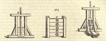
1952. Syphon sluice, As it is practically impossible to form sluices and drains that do not lose more or less water, owing to the great pressure of the volume in the lake or pond, it is better, where the supply is very limited, to have no drain or sluice, and to draw off the water when required by a large syphon, which may easily be formed of boards; or a drain may be formed, and, instead of a sluice, a well of clay adopted as a stopper. The
