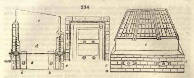
1553. The frame on props, in construction, resembles the Alderstone pit, excepting that the superstructure is a frame instead of masonry. Such frames are much used about London to grow pines, the back being enclosed by walled hurdles, supported by the props as stakes, and round the hurdles linings of dung are applied.
