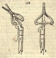
1359. The climbing-spur (fig. 153.) is of two sorts, one with, and the other without a stem. The first sort (a) is fastened to the upper part of the leg with a leather belt (b); the other sort (c) is tied to the feet. By means of these spurs, one on each foot, naked-stemmed trees may be ascended to any height, and when it is wished to stop a short time at any part, the screw of the ring (d) is entered in the trunk, and forms a firm point for one foot. (Lasteyrie, Coll. de Machines, &c.)
