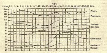
tical lines representing days of the month, and the horizontal ones degrees, the variations of each house, and the open air, may be shown by wavy lines made by daily increments depressed or raised, according to the rise or fall of the thermometer in each separate
