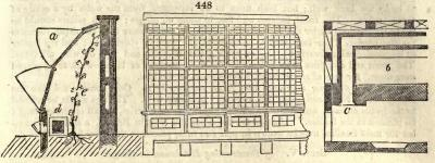
2672. As a peach-house for a main crop, we would suggest a polyprosopic roof, with the sashes (fig. 449. a) opening on the principle of Venetian blinds; the flue (d) may pass round the house, and the trellis (c) be placed between the flue and front glass; both the flues and front glass may be supported on cast-iron props (e). may be forty feet, breadth and height twelve feet.
