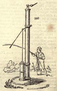
is that which is furnished with a suckingpipe (a), like the fire-engines, by means of which, if there are ponds or regular supplies by pipes or wells in a garden, the labor of carrying the water is avoided.
