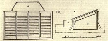
foot or eighteen inches of the glass with  $\tan(a)$ , and heated by an exterior lining if necessary. The tree is planted in a box (b), by which its roots are confined so as to benefit by the heat of the  $\tan$ , and the branches are trained on a trellis (c), close on the bed. Instead of  $\tan$ , dung may be used, covered in the flowering season with earth, or  $\tan$  and earth. In such pits peaches are ripened in Holland, by the middle of May. (Hort. Trans. v. 325.)
