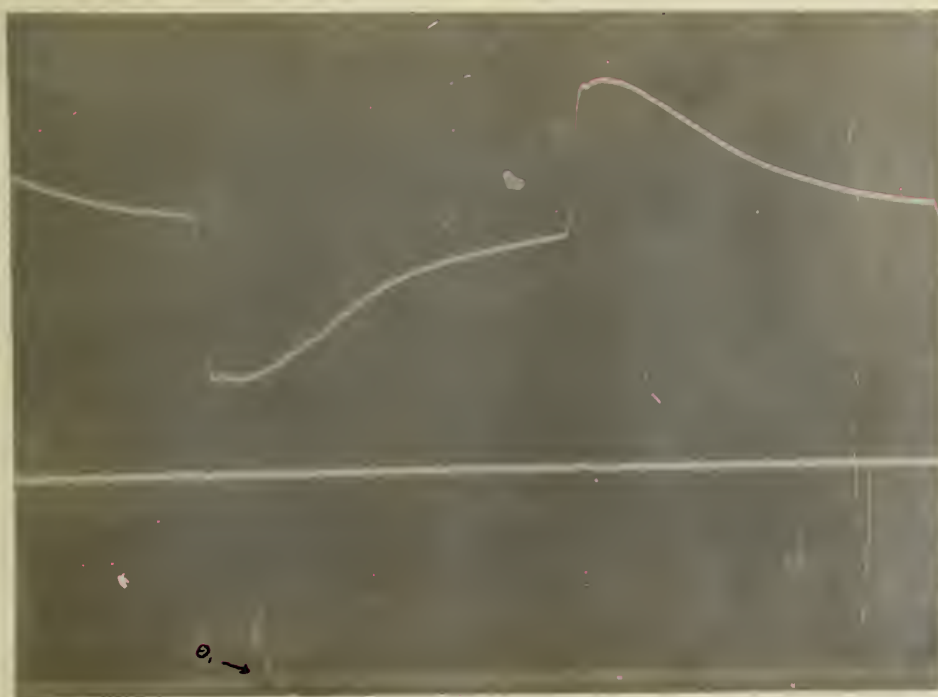
Fig 34 Top curve, Primary Coil current. Middle " , Condenser current. Bottom " , Reference \theta = 0^\circ Point indicated by kick.
