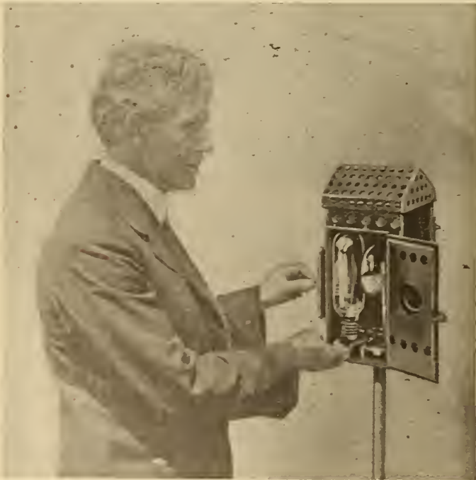
Oscar M. Scheck and His Adapter. This Device Is for Changing Carbon Arc Projection Machines for Use with Mazda Lamps
