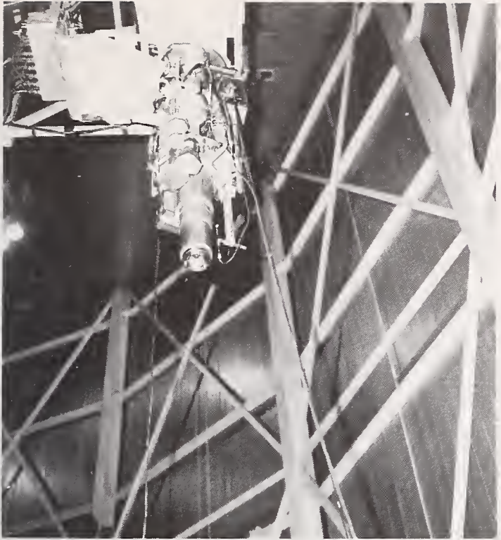
FIG. 5. APRF REACTOR POSITIONED 6 M ABOVE BORATED CONCRETE FLOOR FOR CORE SURFACE LEAKAGE FLUX MEASUREMENT
