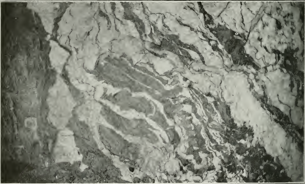
Contact of quartz and schist on the N. W. wall of No. 4 vein, Hollinger mine where vein was intersected in the first cross-cut from No. 1 vein on the 100-foot level. Width of exposure, 6 feet.
