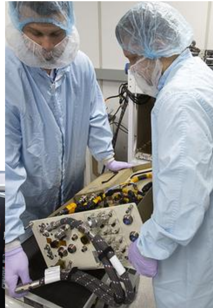
Power Distribution Assembly
