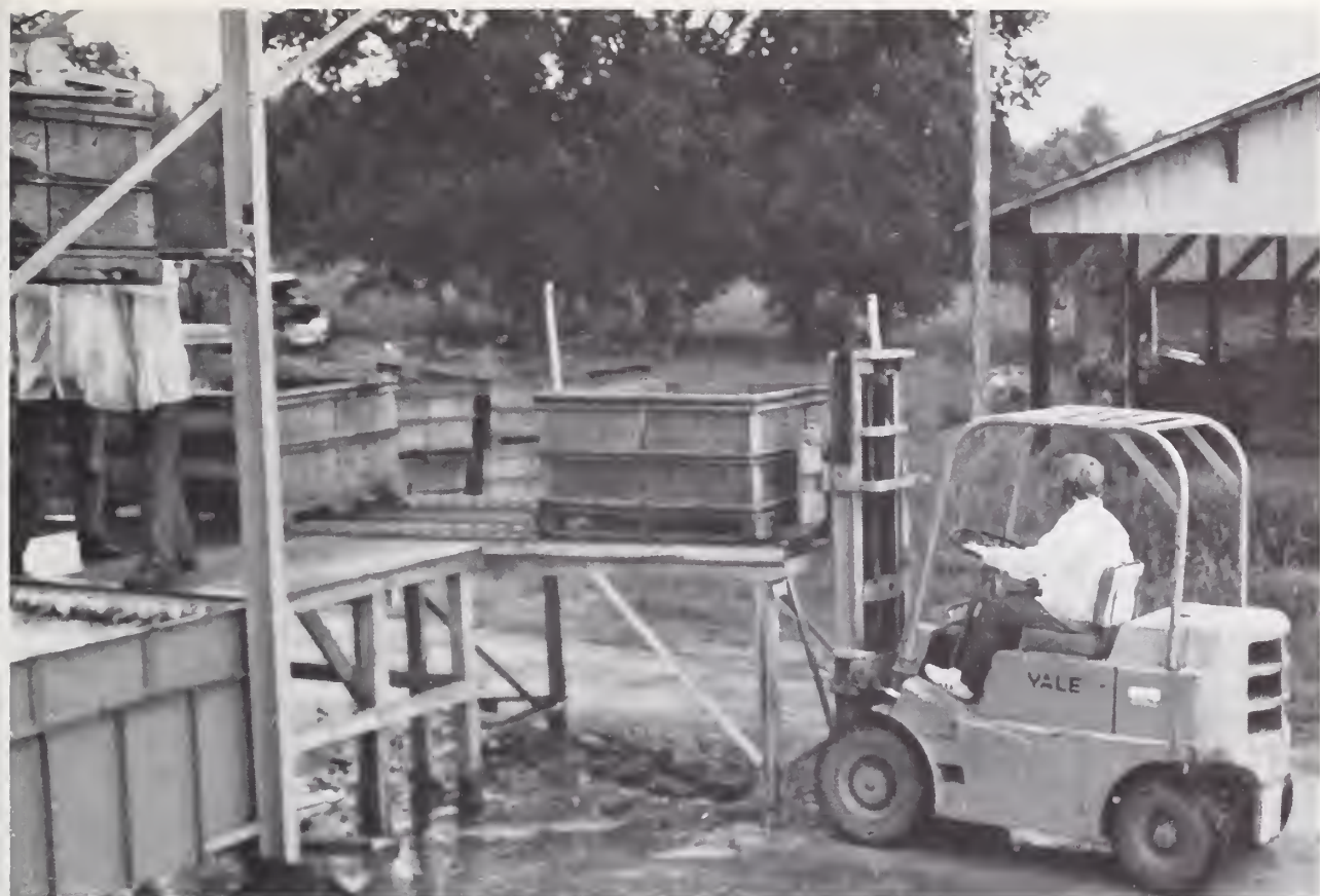
FIGURE 11.—Forklift carries pallet boxes from temporary holding shed to pallet box conveyor.
