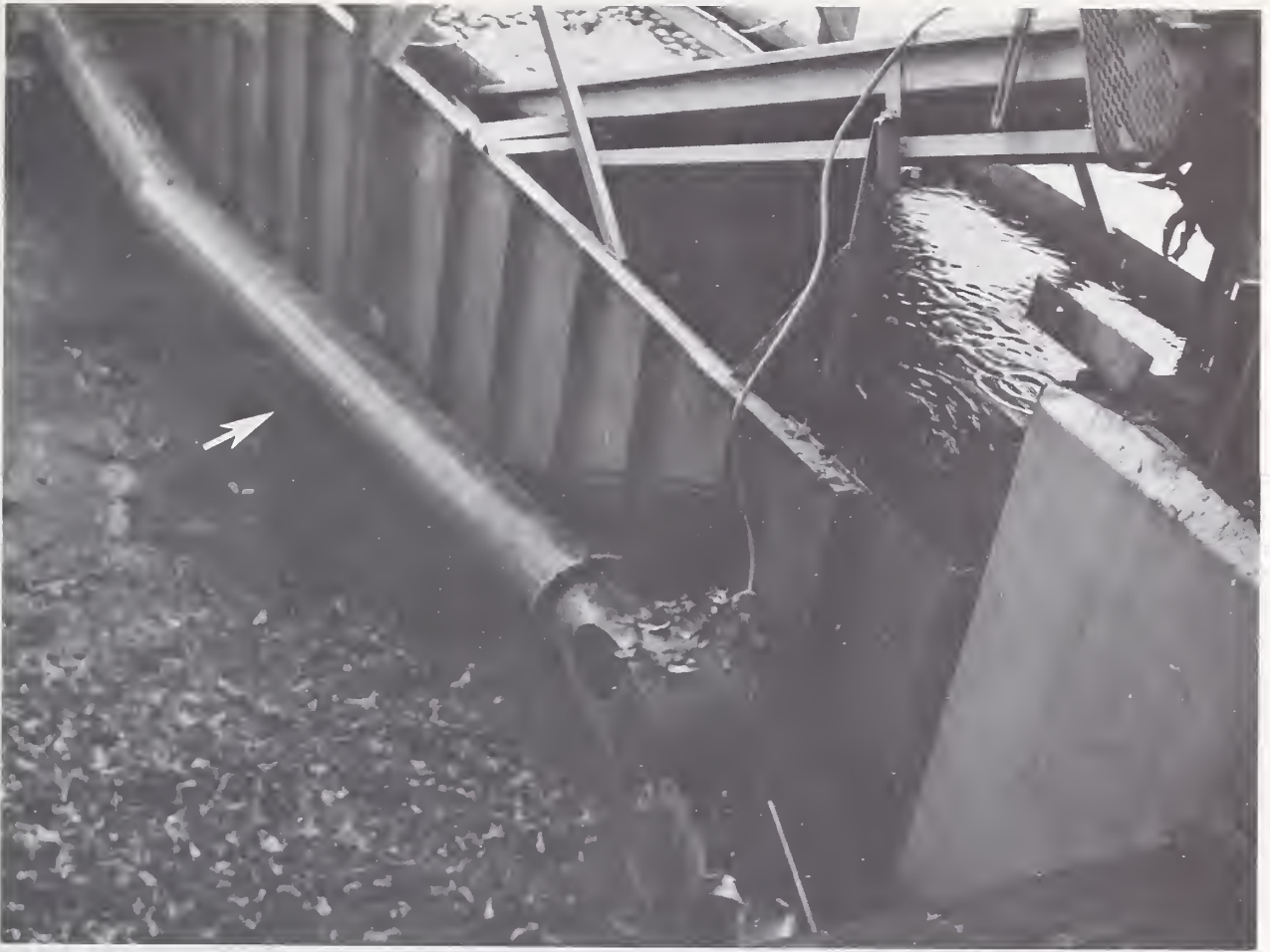
FIGURE 6.—Water is pumped from sump through an 8-inch pipe to distribution manifold in loading end of tank.
