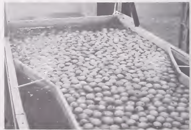
FIGURE 5.—Guide partitions that extend from false bottom to top of tank channel peaches into an area the width of elevated roller conveyor.
