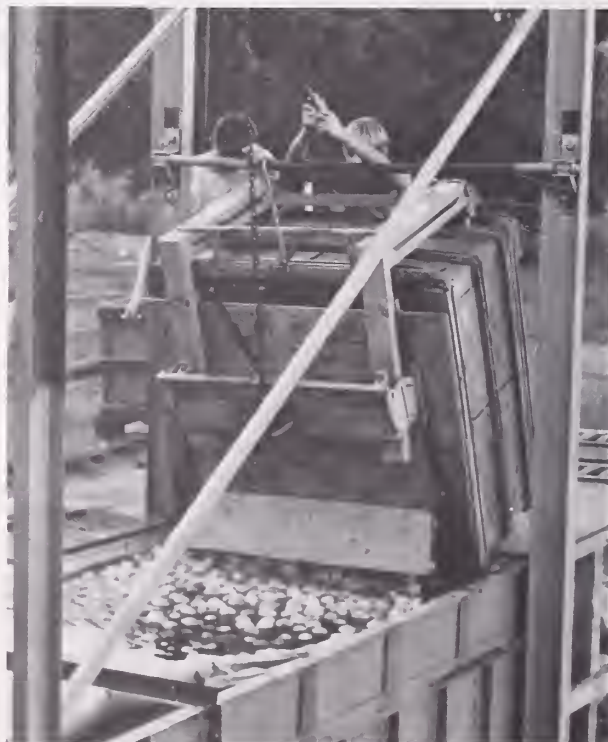
FIGURE 14.—When cage has rotated 90°, the peaches push open hinged discharge door in cover plate and fall into water in tank.
