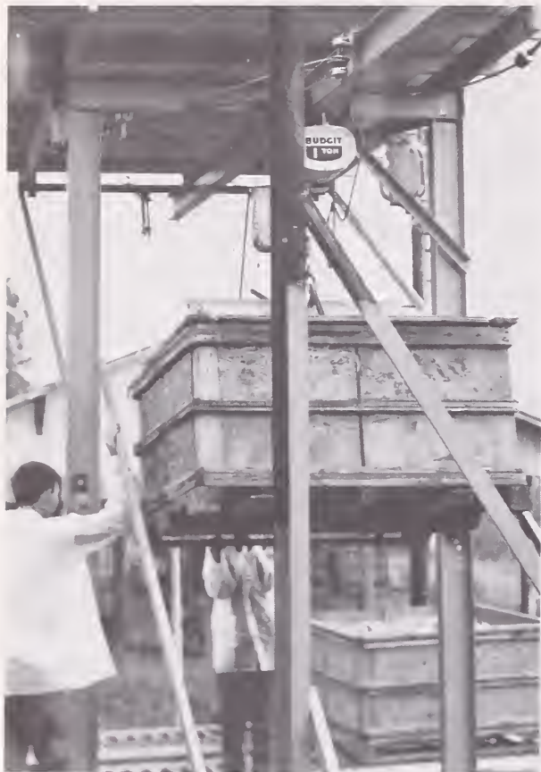
FIGURE 13.—Mobile forklift cage on monorail conveyor system.
