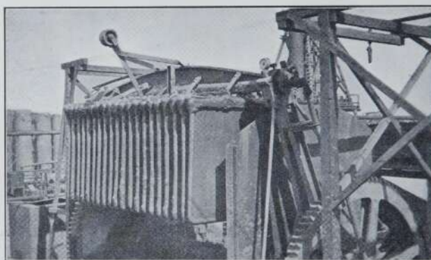
RIDGWAY VACUUM FILTER PRESS FOR SEPARATING GOLD SOLUTION FROM SLIMES, VICTORIOUS MINE, ORA BANDA.
