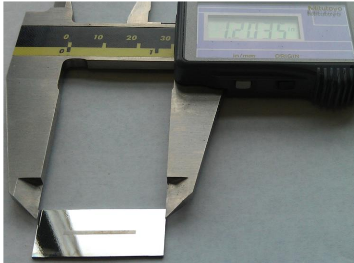
Figure 15. Diffusion couple coupon after sectioning and polishing as received from Sandia National Laboratories.
